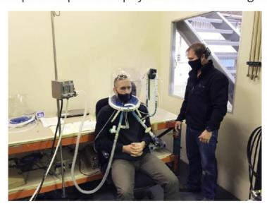
The design of the Air-Oxygen gas blender unit incorporates two easily adjusted air and oxygen flowmeters. The required FiO2% (Oxygen %) is easily set by adjusting the two flowmeters to a Flow Meter Settings Card provided. The system facilitates stoppages in treatment with the provision of a hood supply isolation valve and the top of the hood is easily detached and removed without needing to remove the neck seal and neck ring.
